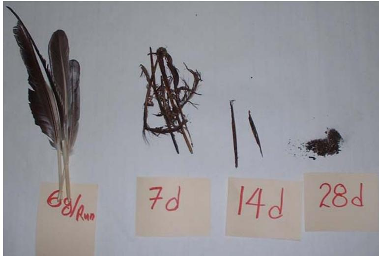
Figure 1. Illustration of the fate of goose feathers in a thermophilic biological treatment system.
