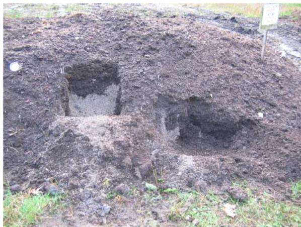
Figure 7. Photograph of Pile #3 following 3.5 inch rain event. Excavation on left depicts penetration of precipitation approximately 12 inches into pile, whereas excavation on right shows saturation of pile base from surface water impacts.
