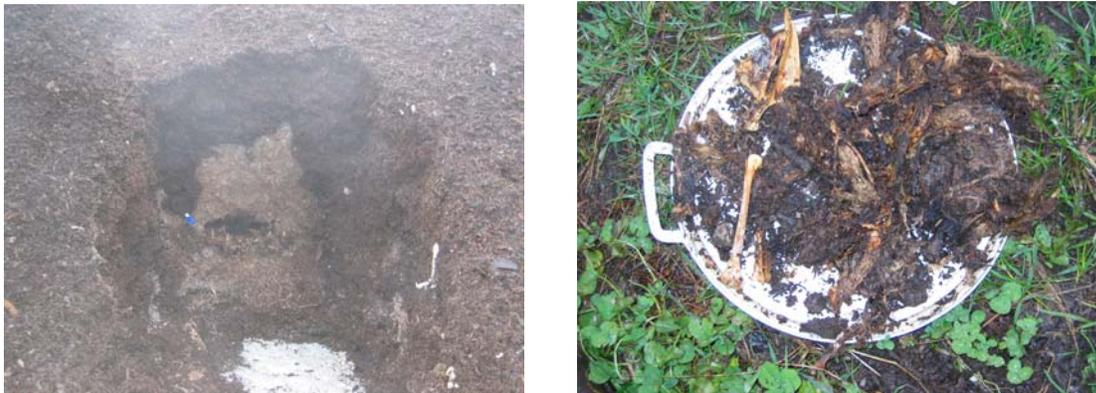
Figure 6. Photographs depicting sludge-based compost pile at day 35. Photograph on left shows pile cross-section (note: blue-tipped pen has been placed adjacent to single bird layer); photograph on right shows clean, brittle bones and dry, charred feathers.
