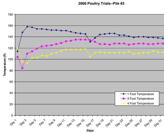
Figure 3. Summary of one-foot, three-foot and four-foot temperatures recorded in Pile #1-#3 during the 2006 poultry trials. Note consistent temperature performance among the individual trials.
