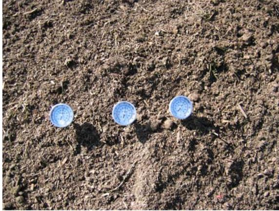
Figure 1. Photograph depicting temperature sampling array of thermometers placed (from left to right) at one-foot, three-foot, and four-foot depths.
